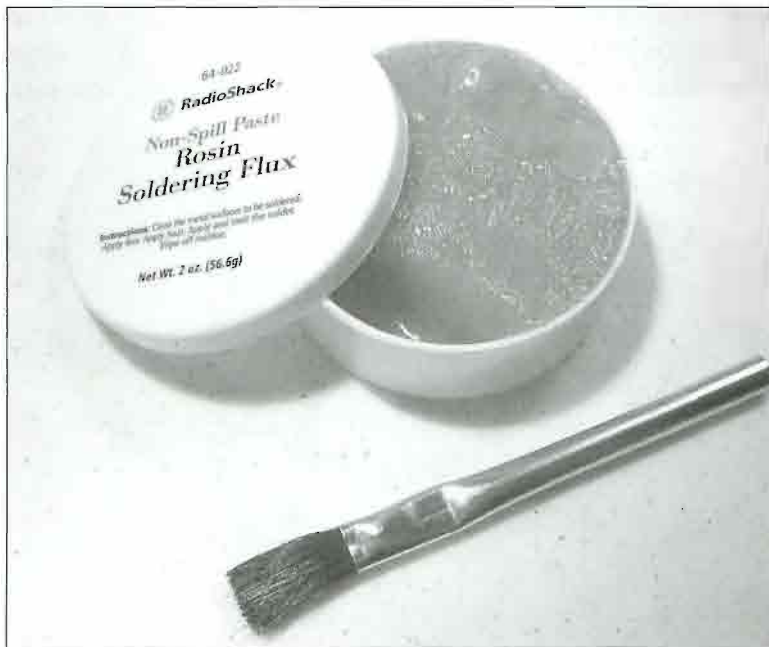
FIGURE 6.20 Rosin flux is a necessity when soldering!
