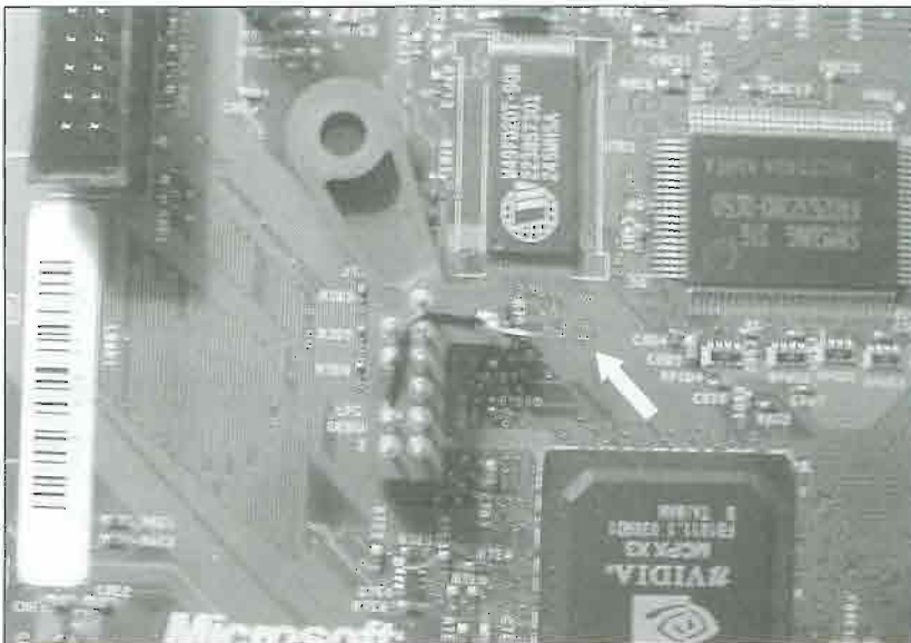
FIGURE 5.12 Seating the D0 pin into the D0 point on the motherboard.
