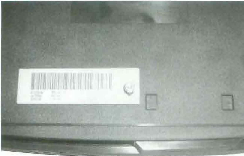
FIGURE 2.14 Two screws are hidden behind labels.
