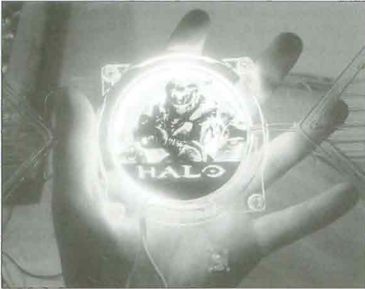
FIGURE 13.6 Close-up of the cold cathode shining through the custom jewel.
