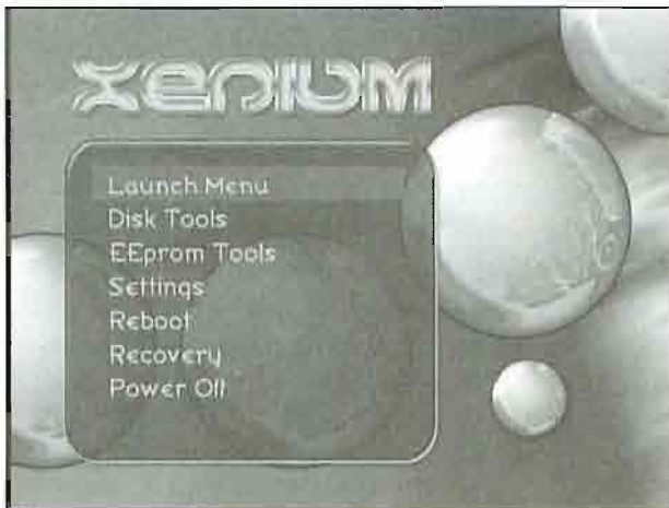
FIGURE 1.8 The Xenium O/S 2.0 (built into the mod chip's BIOS) is used to run custom Xbox software.
