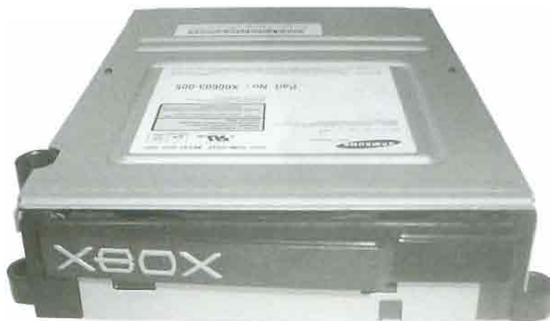
FIGURE 11.20 The front tray panel on the DVD-ROM drive.
