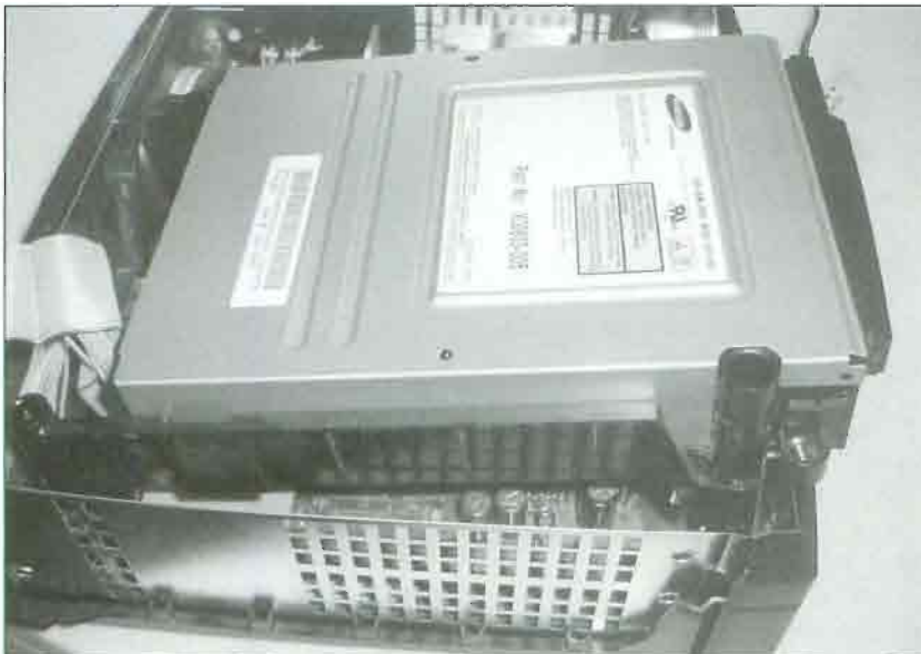
FIGURE 2.39 Lifting the DVD-ROM drive and tray out of the Xbox case.
