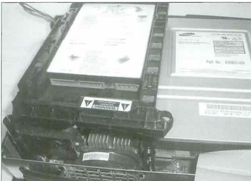
FIGURE 2.29 Lifting the hard drive tray out of the Xbox case.
