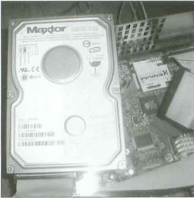
FIGURE 1.9 You can replace the stock Xbox hard drive with a new model with 30 times the capacity.
