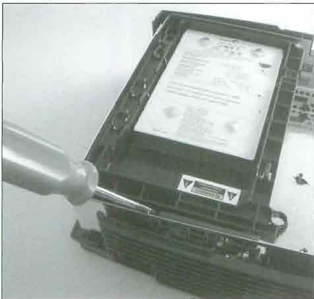
FIGURE 2.28 Removing the hard drive tray may require the help of a screwdriver to pry it up.
