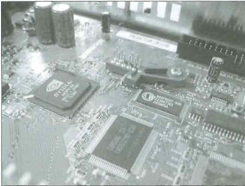
FIGURE 5.13 The solderless adapter has been screwed down to the motherboard.
