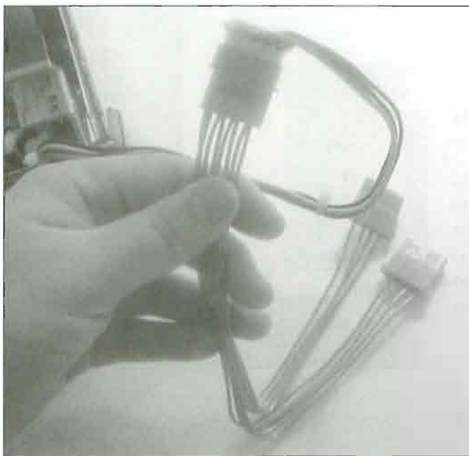
FIGURE 12.8 The Y splitter is connected to the power cable.
