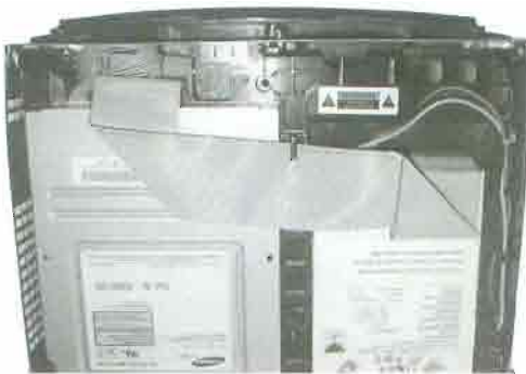
FIGURE 2.22 The IDE cable is routed carefully underneath the cover.
