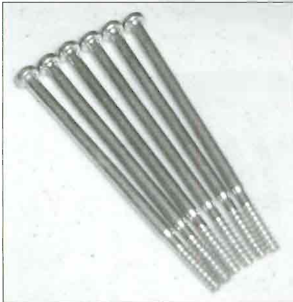
FIGURE 2.16 The six Torx-head screws that keep the Xbox together.
