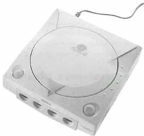
FIGURE 1.4 Sega Dreamcast was a very capable video game console that was powered by Windows CE and DirectX.
