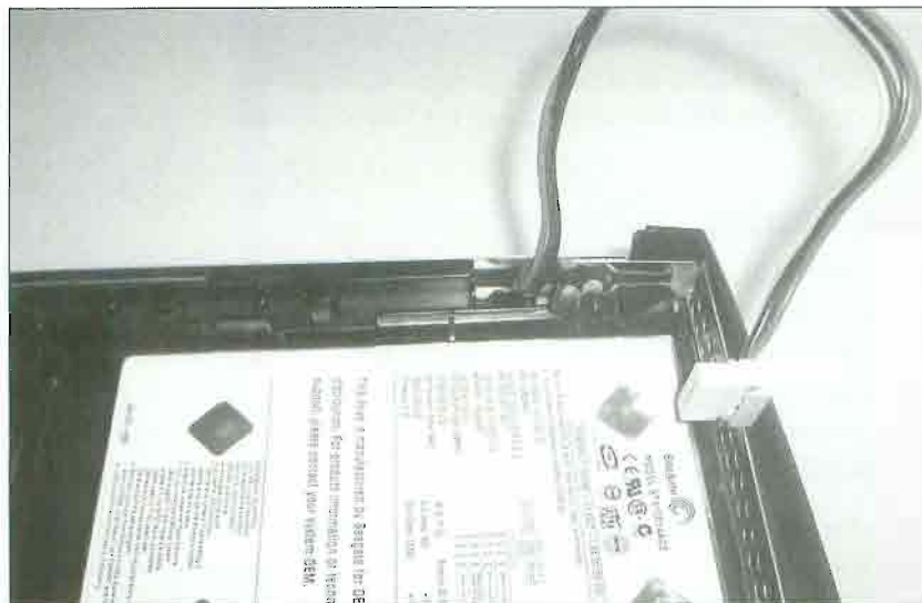
FIGURE 2.26 Freeing the power connector from the hard drive frame.
