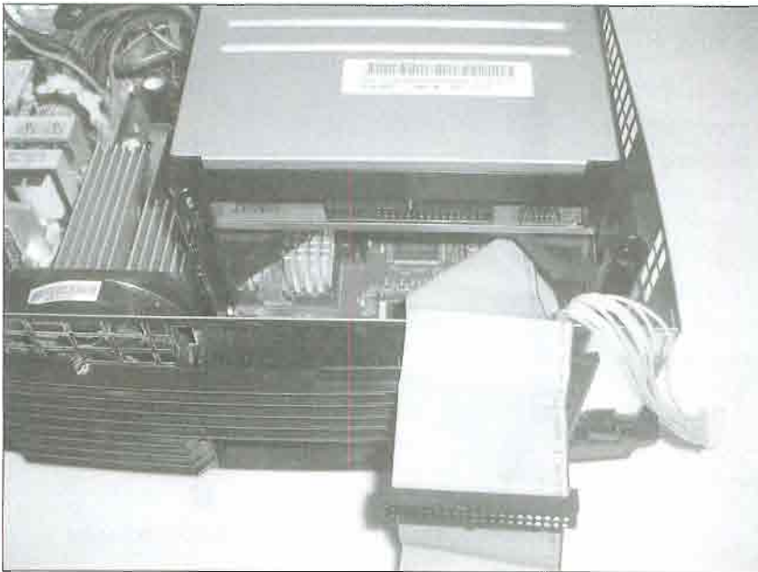
FIGURE 2.38 Moving the cables out of the way.
