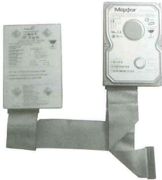
FIGURE 12.6 Installing the IDE cable on both drives.
