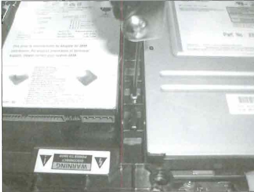
FIGURE 2.24 Removing the single screw holding down the hard drive frame.
