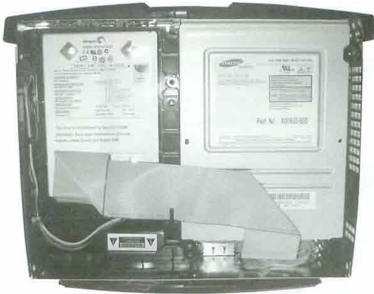
FIGURE 2.21 The drives are connected to the motherboard with a standard IDE cable!
