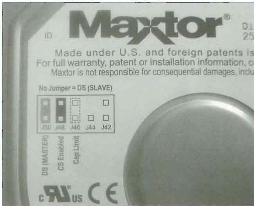
FIGURE 12.5 Master/slave settings for the new Maxtor drive.
