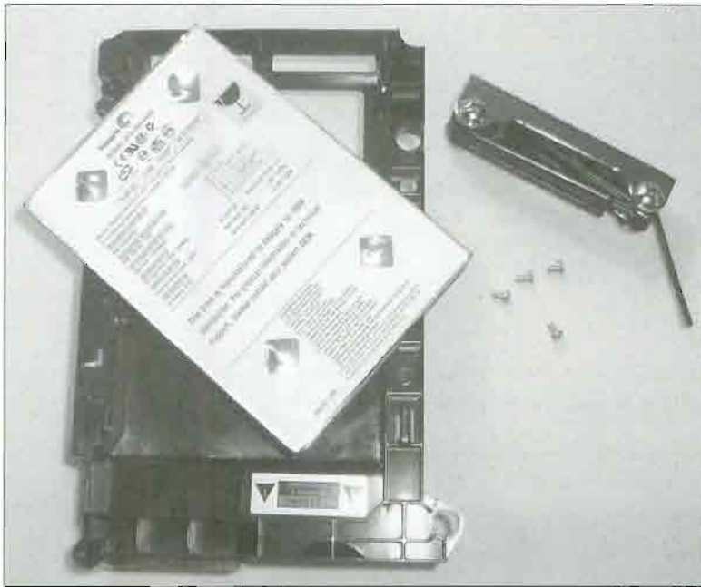
FIGURE 2.32 Removing the hard drive from the tray.
