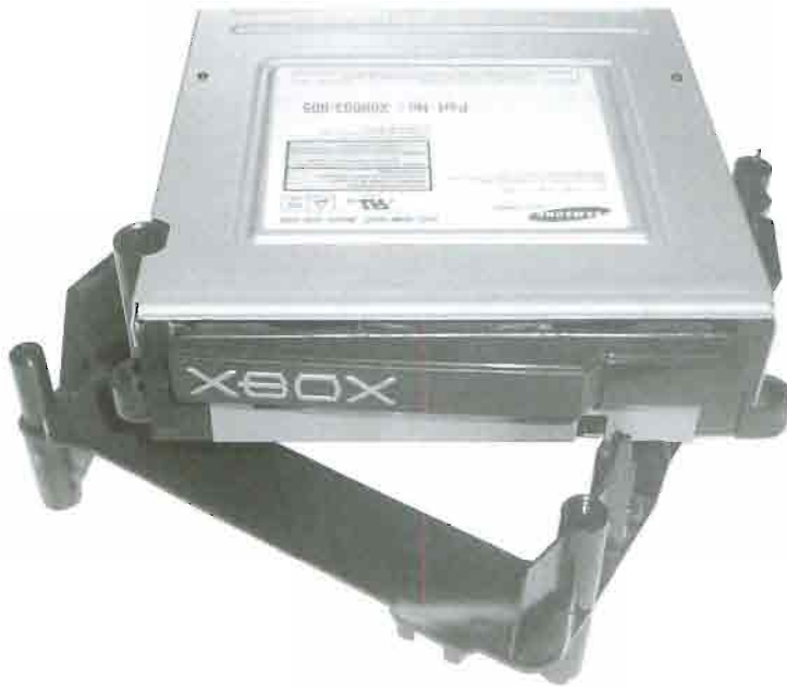
FIGURE 2.41 Disengaging the DVD-ROM drive from the tray.
