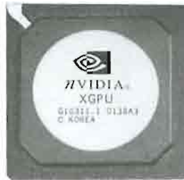
FIGURE 2.10 The Xbox graphics processor.
