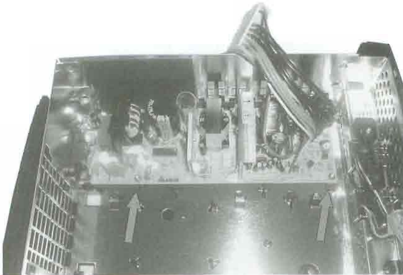
FIGURE 11.12 The Xbox power supply is held in place by two Torx screws.
