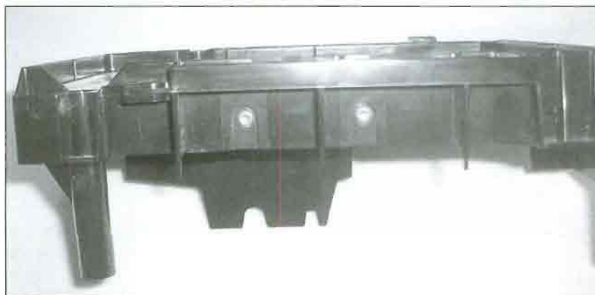
FIGURE 2.30 The hard drive screws on the left side of the tray.
