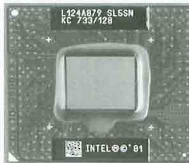
FIGURE 2.9 The Xbox central processor.
