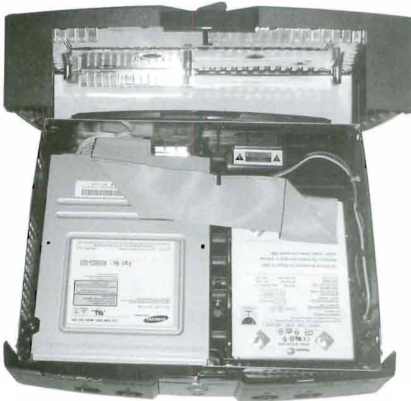
FIGURE 2.20 The top portion of the Xbox case has been removed.
