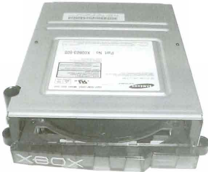
FIGURE 11.31 The new tray has been installed on the DVD-ROM drive.
