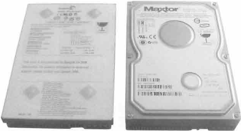
FIGURE 12.3 A stock Seagate 10GB hard drive next to a new Maxtor 250GB drive.
