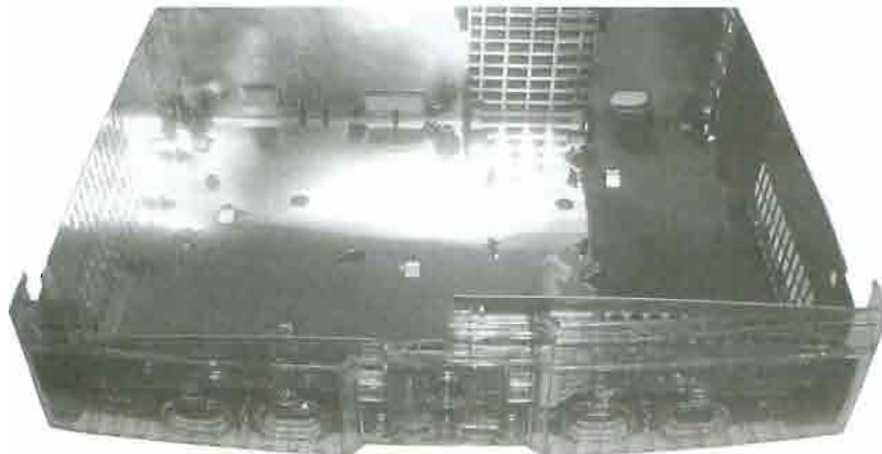
FIGURE 11.38 The clear front panel has been installed on the case.
