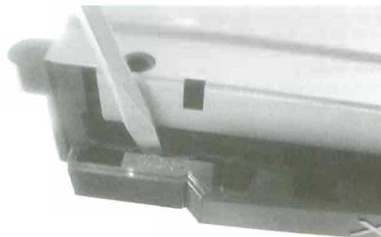
FIGURE 11.21 Releasing the front tray panel with a screwdriver.
