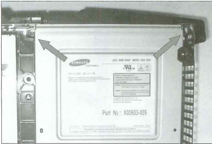
FIGURE 2.33 The two screws holding down the DVD-ROM frame.
