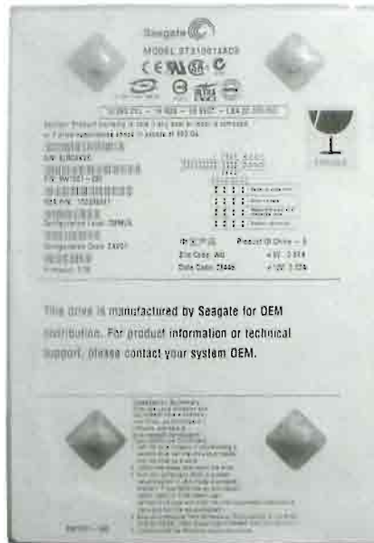
FIGURE 2.8 The Xbox hard drive (typically 8GB).
