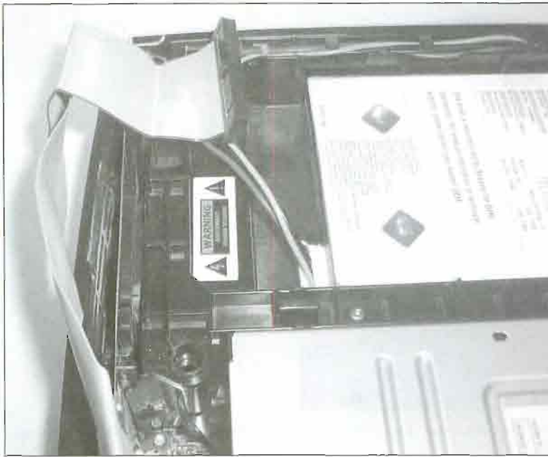
FIGURE 2.27 Unplugging the IDE cable from the hard drive.
