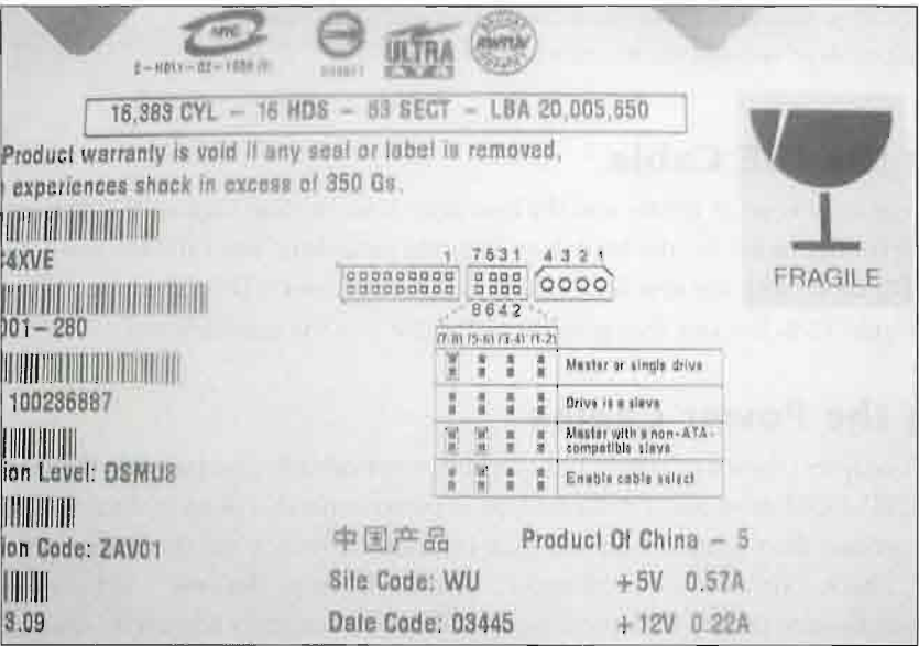
FIGURE 12.4 Master/slave settings for the stock Seagate drive.
