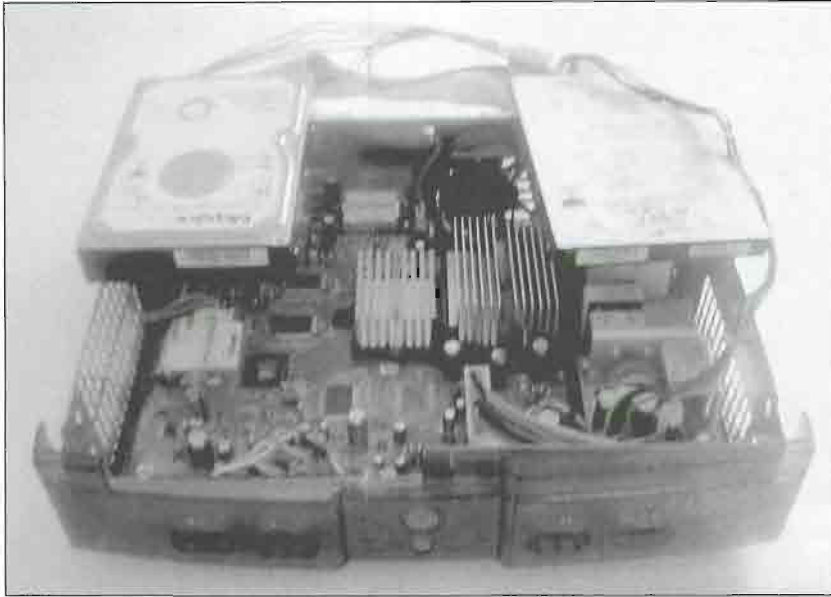
FIGURE 12.10 View of the dual hard drive setup from the front.
